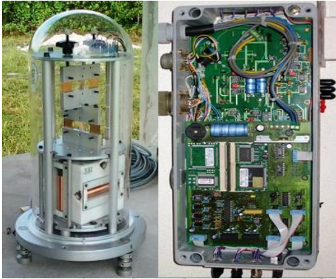
Fig.2.4a: Left -suspended block of fluxgate sensor Right-MAGDALOG data logger. Quantity 2
