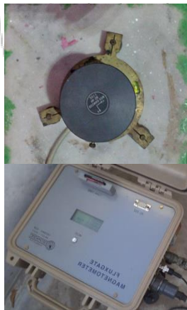
Fig.2.4a: Left -suspended block of fluxgate sensor Right-MAGDALOG data logger. Quantity 2
