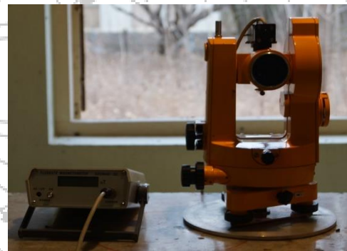
Fig 2.4l: THEO-020A & GEOMAG-03 absolute magnetometer for field stations
