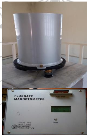
Fig. 2.4e: GEOMAG-02MO upper-sensor, lower-electronics. Quantity 1.
